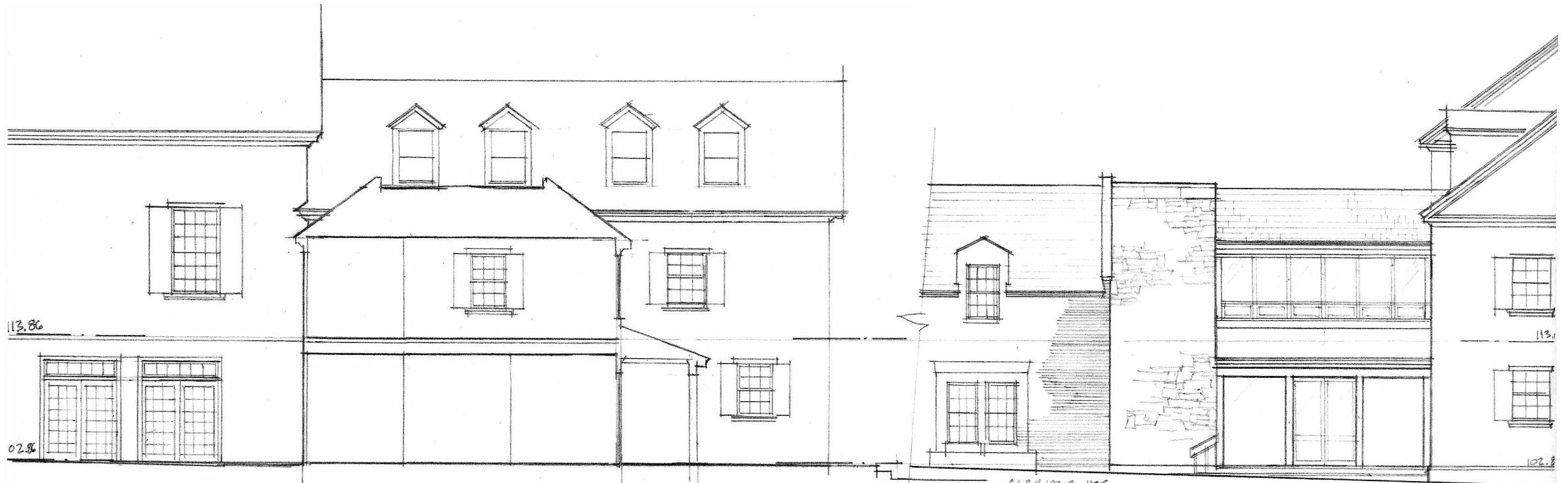
WEST ELEVATION / LINK SECTION
