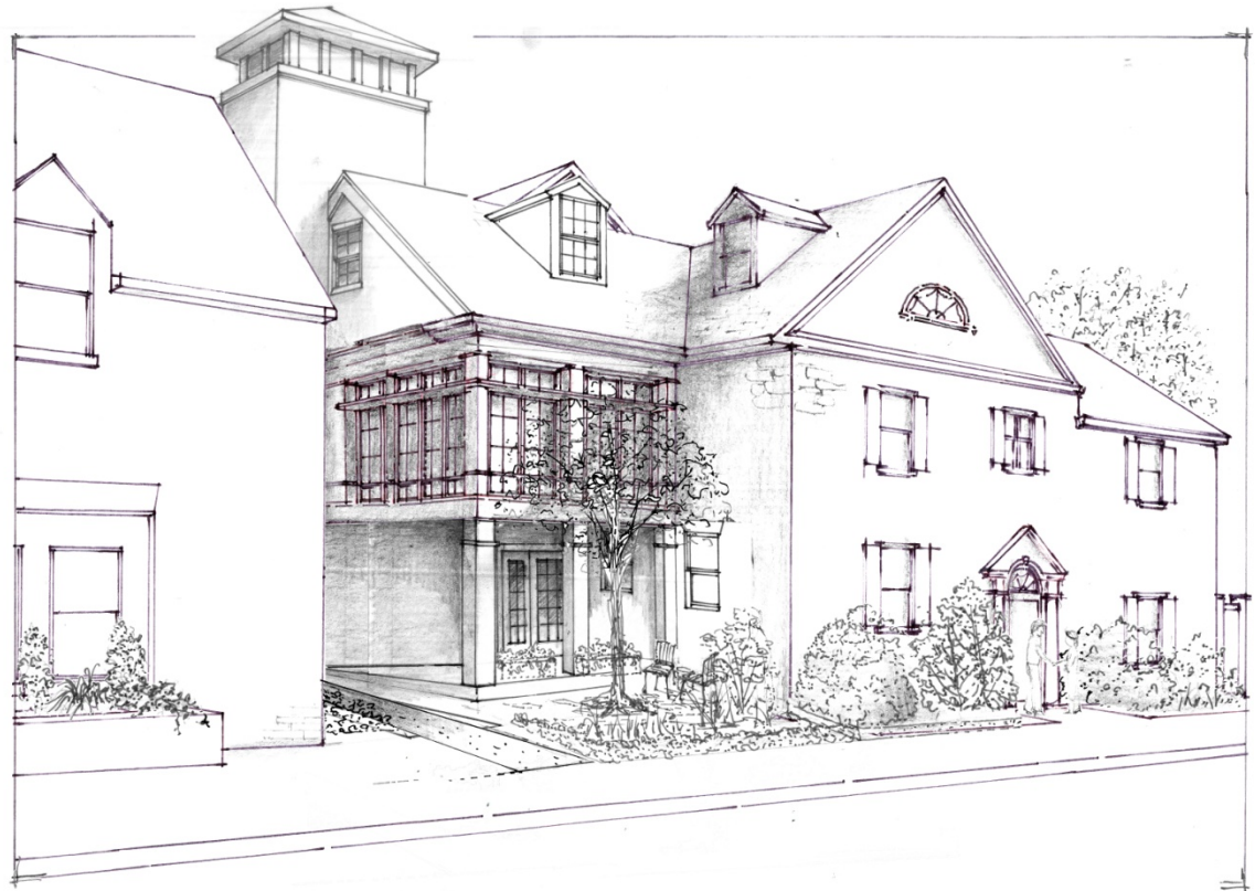
Perspective from Decatur Place. The existing Meeting House is on the right, the new west addition is in the center. A new iron fence and gate, with new signage is proposed along the sidewalk. The old entry door will only be an emergency exit.
